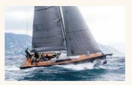
**ADVANCED A44** €650,000 (C£548,000) European Yacht of the Year in 2015, this speed machine has a stylish interior. The hull is GRP with carbon reinforcement and carbon rig. It is pitched as a daysailer, but would serve for short cruises. advancedyachts.it
