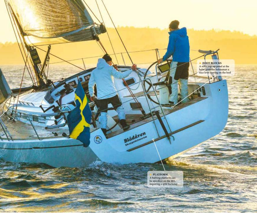
easily reach the German mainsheet on manual winches just ahead on the coaming. The mainsheet track is recessed into the cockpit just ahead of the pedestals, and we found it easier to spill wind in the gusts using the traveller itself.
