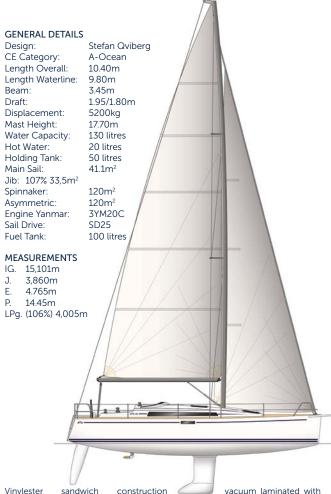
Vinylester sandwich construction vacuum laminated with multiaxial glass fabric, core material is 20mm Divinycell, solid laminate around keel, rudder and through hull fittings.
